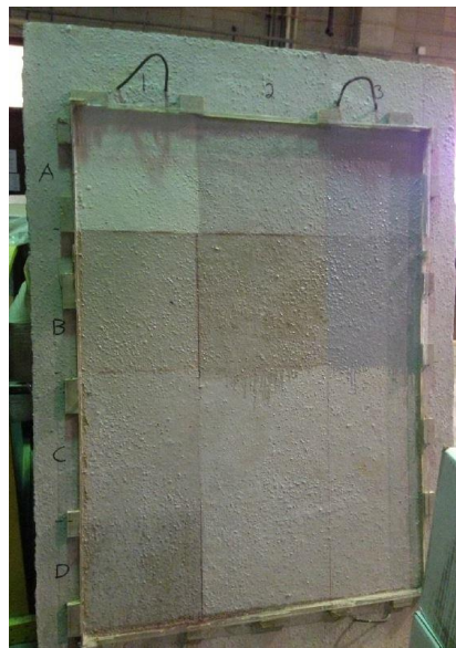
Fig. 5- Coating treatment application on a ponding slab [43].
